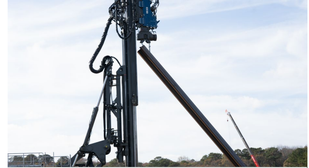
Quieter Machine for Temporary Sheet Piles (shoring of sandy soil)
